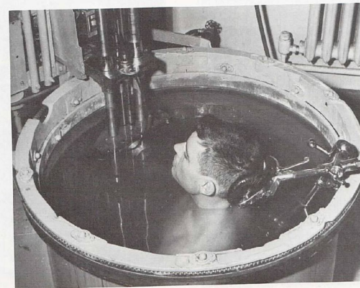
Fig. 1-3. Scanning position for transverse cross-section of the neck. The 2 1/2-inch focused transducer is seen just below the water level. The transducer carriage travels around the tank on the outside track.
